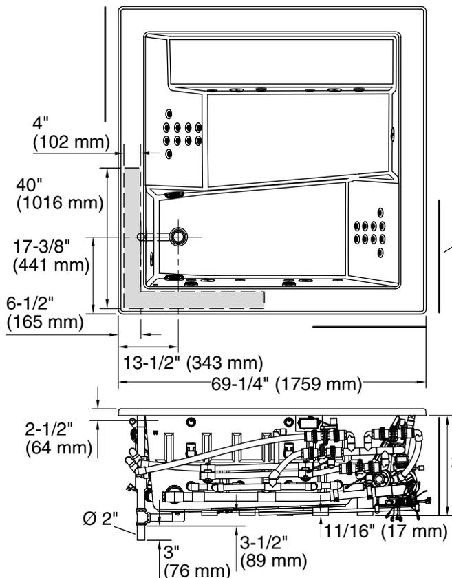
No change in measurements with drain shown. (K-7167-AF or K-7167M-AF)
