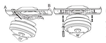
Place the left tab (A) of the lower mountingbracket into a left large slot (A) in the uppermounting bracket. Then slide the right tab(B with Oval Hole) of the lower mountingbracket into the right large slot (B) on theupper mounting bracket until all four holesare in alignment. (PS: A tab is for A slot, and B tab is for B slot)
