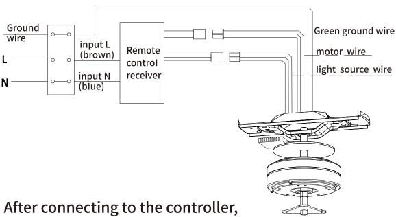
After connecting to the controller, install the main body of the fan and lock the security screw.
