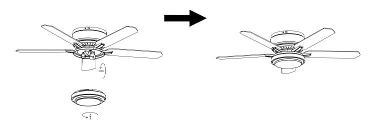
instsll the lamp shade in place and rotate the lapmp shade clockwise.
