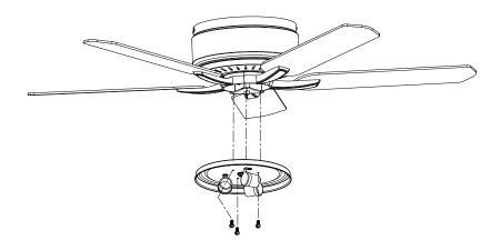
Connect the wire from the bottom of the fan motor assembly tothe wire from the light kit pan. Attaching the light kit to the fan motor. Make sure all the screws are firmly tightened. (Bulbs not included)
