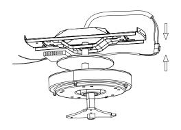
Safety rope installation procedure
