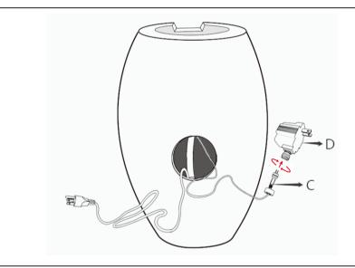
Connect the end of 6 Led Light(C) into Transformer( D).
