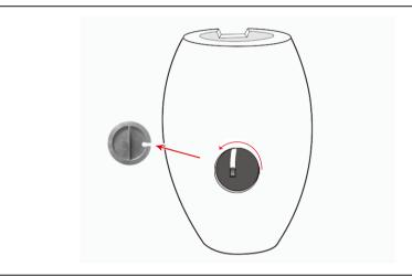
Place the Fountain Body(A) on a level surface away from areas where it is likely to get colgged with leaves and make sure that the cable will reach the socket and open the back door(anticlockwise).
