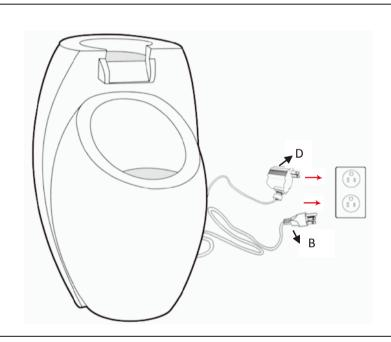
Plug the Pump(B) and Transformer(D) to the socket. Then the water will start to flow in minutes.
