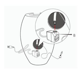
Insert water pipe into the Pump(B).
