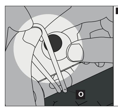
The Cover/Tarp J is secured onto the structure using bungee ball O. Use one bungee ball per grommet on the tarp. Notice that, at the four corners, use two bungee balls for one grommet.
