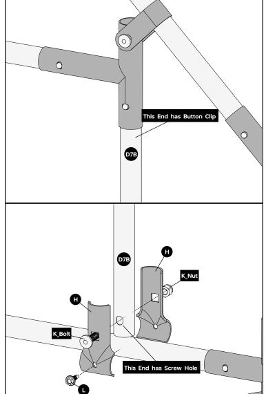
Tube D7B has two different ends. Use the end with screw holes as the bottom end. For screw L, you will need a power tool to drive it into tubes.
