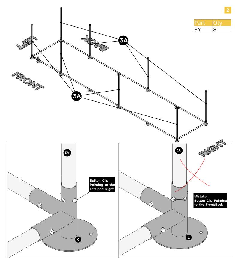
There are two pairs of holes on the vertical tube of Part C. When connecting 3A to Part C, make sure that the Button Clip is pointing to the left and right. An incorrect layout is also shown above.
