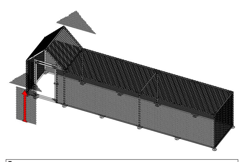
For the net used in this step, it's easier to measure and cut the net, and then fasten the cutted net to the tubes.
