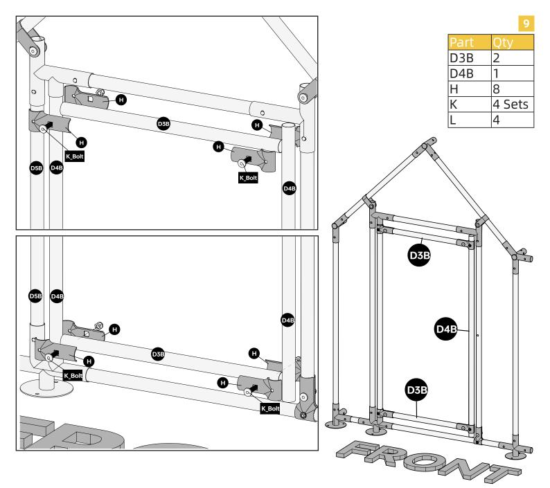
Do not worry too much about the exact location of D3B and D4B. Just make sure D4B is completely covered by the two pairs of H.
