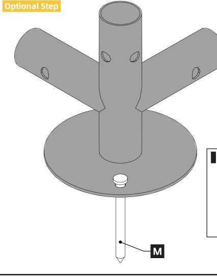
When you feel like you have chosen a perfect spot for your chicken run and do not plan to move it, you can fasten it to the ground using the anchor M.
