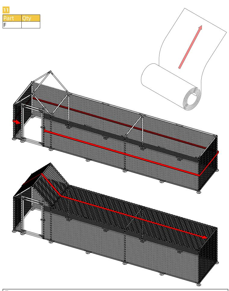
In the package you will find the poultry net. When attaching the net to the chicken run structure, do not precut the net. Instead, roll the net along the tubes and cut it. The arrows on the illustrations indicate the flow of the net. Follow the arrows to roll and cut the net. Use zip-ties to fasten the net to the tubes.
