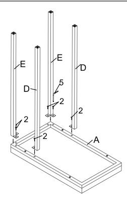
Step 2: Attach Front/Back Metal Bar (D, E) to Top Frame (A) by using Short Bolt (2). Secure with an Allen Key (5). Do not fully tighten all bolts at this stage.
