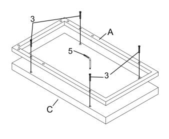
Step 1: Attach Top Frame (A) to Table Top (C) using Screw (3). Tigthen with an Allen Key (5).
