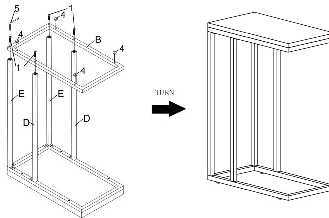
Step3: Insert Cap (4) into the holes of the Bottom Frame (B). Attach Front/Back Metal Bar (D, E) to Bottom Frame (B) by using Long Bolt (1). Secure with an Allen Key (5). Fully tighten all bolts at this time.
