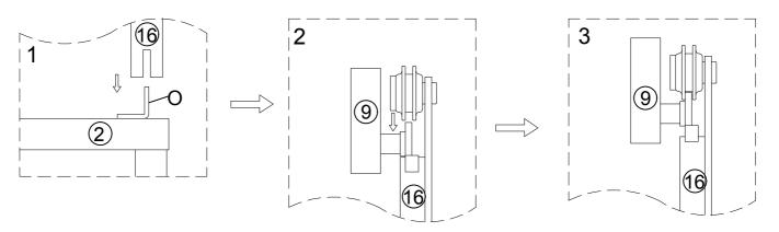
Part 2--Bottom frame Part 9--Door track Part 16、17--Sliding door Part O--Angle bracket
