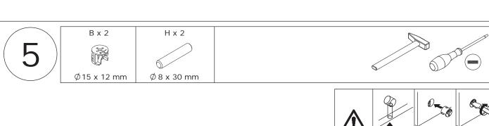
Attach board 3 to board 15 with wooden dowel(H) and turn cam lock(B) clockwise to tighten as shown.
