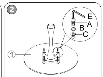
a)With assistance, lay Table-top (1) flat with the bottom-side facing up on a material that does not scratch or damage the part.
