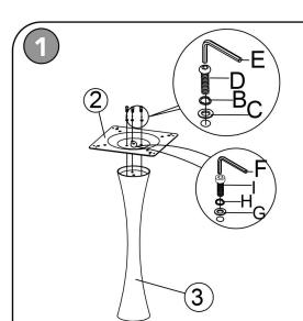
a)Position Leg (3) and Top Plate (2) as shown and align screw holes on both parts.
