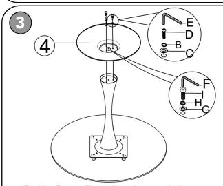
a)Position Bottom Plate (4) as shown and align screw holes on (4) to the screw holes on the leg. b)Use Screw (D) fitted with Spring Washer (B) and Flat Washer (C) to fasten (4) to (3). Use Allen Key (E) to drive (D). Do not tighten (D) completely until all 3 screws are in place.
