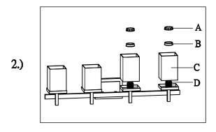
Step.2: Use the socket ring (A) & (B) to secure glass (C)on socket (D).
