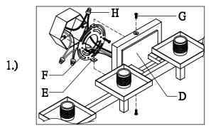
Step.1: Remove mounting bracket (E) from fixture and install to electrical box.
