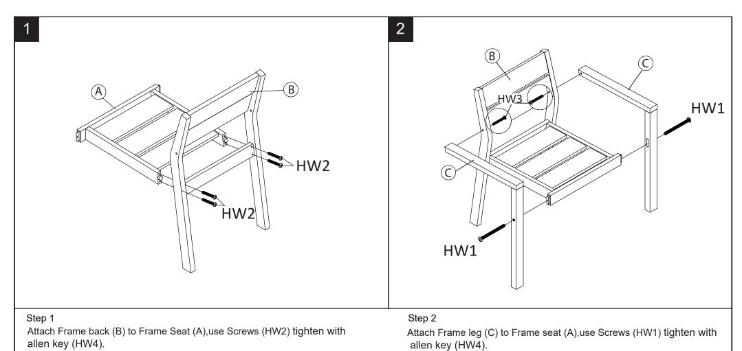
Attach Frame back (B) to Frame leg (C),use Bolts (HW3) tighten with
