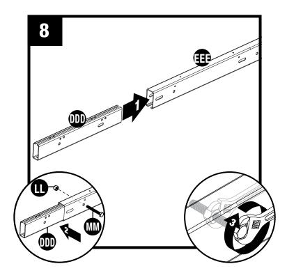
Place ridge beam joiner (DDD) into the 3' ridge beam (EEE). Secure with hex bolt (MM) and nut (LL).
