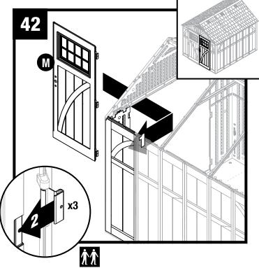
With door hinge in open position, slide one door hinge over each hinge receptacle on inside of right front panel.
