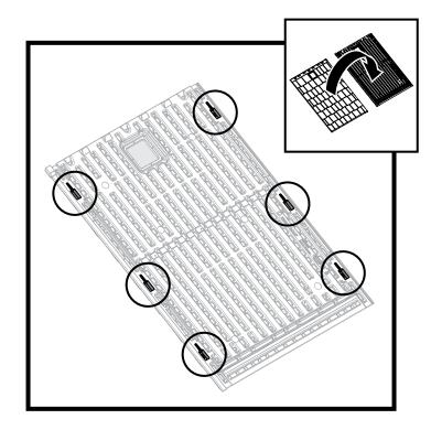
Before proceeding, locate and identify the six slots on interior side of right and left roof panels.
