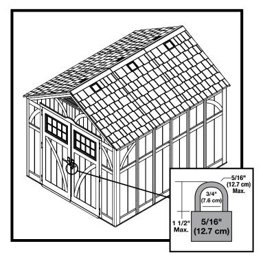
Attach a 5/16" lock (not provided) to door handles, to properly secure shed.
