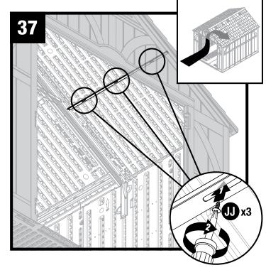
Secure roof support to roof using three screws (JJ).
