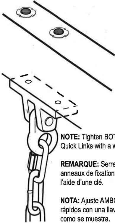
**NOTE:** Tighten BOTH Quick Links with a wrench
