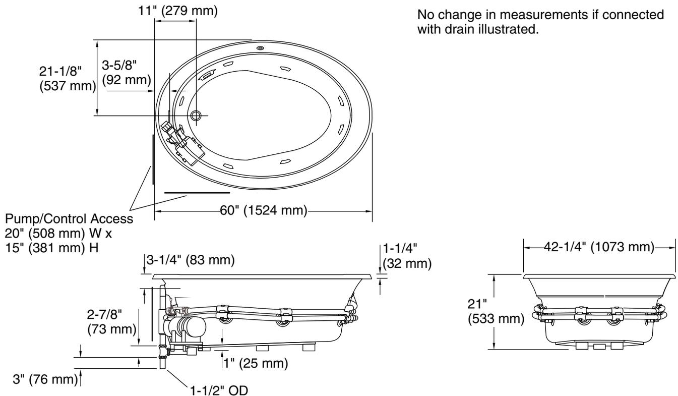
No change in measurements if connected with drain illustrated.
