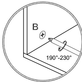
4. Rotate cam(s) clockwise 190°-230° to lock panels together
