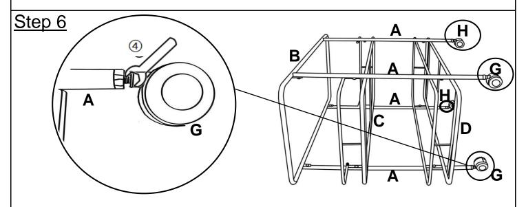
Attach Wheels with Brakes(H) to Legs(A) in Left side using Spanner(4). Attach Wheels(G) to Legs(A) in Right Side using Spanner(4).
