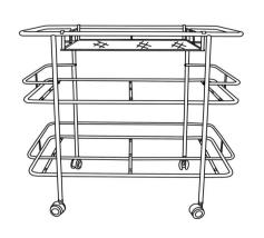
Attached Top mesh Shelf (F) to Pre-assembled Frame(A,B,C,D,E).
