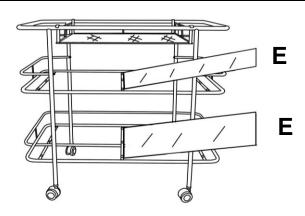
Carefully, insert Glass(E) into Middle Shelf Frame(C) and Bottom Frame(D). Gently press down on the Glass Shelves after you put them into the frame. Please pressure down on each corner to adjust the gap between glass and frame.
