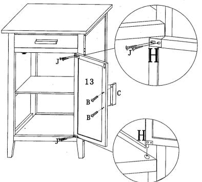
Assemble the Door Pin(H) to one side of Door Panel(13) by using Screw(J), then insert to assembled unit as shown.
