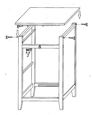
Assemble the Top Panel(5) to assembled unit as shown by using Allen Bolt(E). Assemble the Magnetic Catch(F) to Upper Front Rail(8) by using Screw(J).
