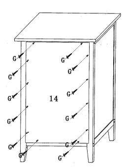
Assemble the Back Panel (14) to assembled unit by using Screw (G) as shown.
