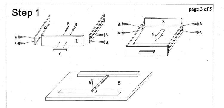
Assemble the Drawer Side Panel(2) to Drawer Front(1) as shown by using Screw(A), then assemble the Handle(C) to Drawer Front(1) by using Handle Bolt(B). Insert the Drawer Bottom Panel(4), then assemble the Drawer Back Panel(3) by using Screw(A) as shown.
