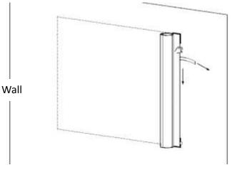
7. Continue removing the entire tape film on the rest of the tape strips one by one.
