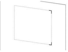
3. Peel off one side of the double-sided adhesive film tape and apply it from top to bottom (vertically) every four to six inches apart from one end to the other.
