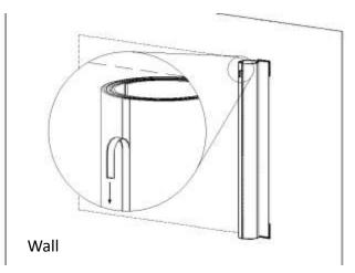
8. Unroll the material to the left and firmly attach the Insta-DE to the installation area until you've reached the other end. Make sure that the material has completely rolled out perfectly flat.
