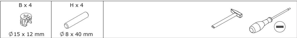
Attach board 6 and 7 to two board 10 respectively with wooden dowel(H) and turn cam lock(B) clockwise to tighten as shown.
