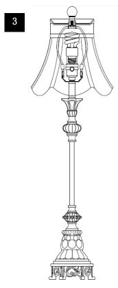
Step 1 Screw the Tube (B) onto the Lamp base (A), Then screw clomn (C) onto Tube (B), Be careful not to twist the power cord and tighten securely
