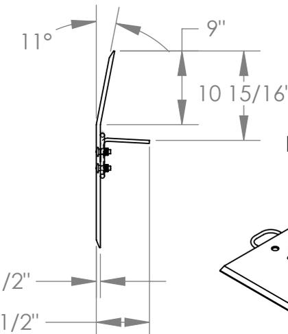
NOTE: BEND OR CROWN IS 11° AND LOCATED 9" FROM EDGE OF DOCKPLATE
