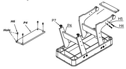
5.Lock the table in the upright position by loosening the handle bolt, folding the table in place, tightening the handle bolt and inserting the bolt (*H3*) and washer (*H5*) as shown.
