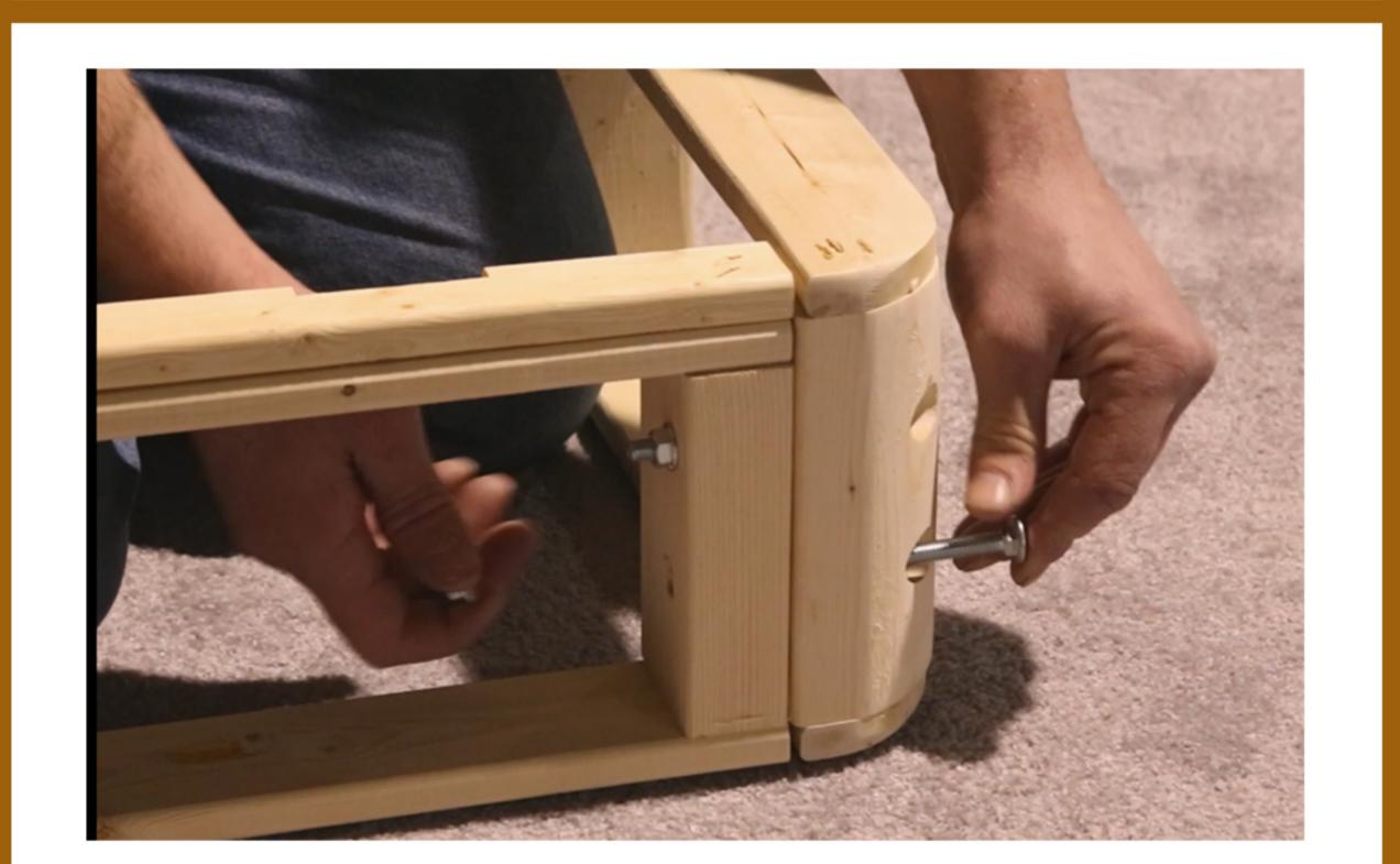
5. Use bolts and nuts to connect long rails to the end rails.
