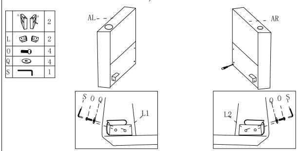
Step 2 Put the screws into the holes one by one. Please do not lock any one of the 3 screws before they are all aligned. After aligning them all and then tighten them with an electric screwdriver.
