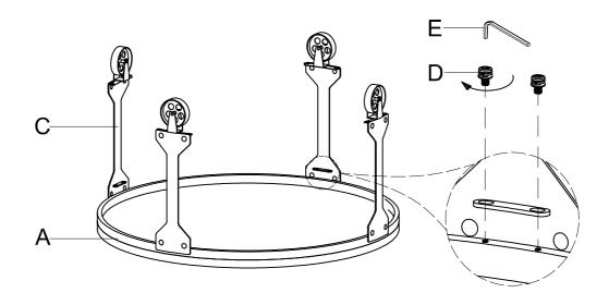
2 Attached lower frame(B) with bolts(D) by allen wrench(E).
