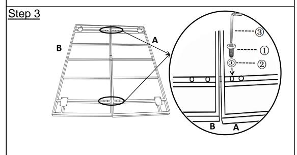
Repeat Step 2 ,Attach Support Bar(C) to Table Top(A) using Bolts(①) and Washers(②) with Allen Key(③).
