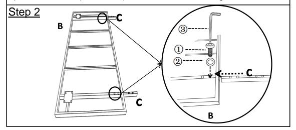
Turn the Table Top Right(B) face down on a clean, non-marring surface. Attach Support Bar(C) to Table Top Right(B) using Bolts(1) and Washers(2) with Allen Key(3).
