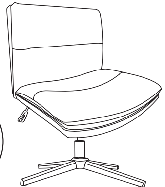
4.Rocking Adjustment Function The tighter the knob is turned, the less shaking it is, and vice versa
