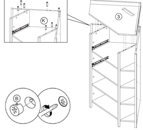
Assemble the left, center, and right decoration strips (4, 5, 6) to the underside of the top panel (3).
