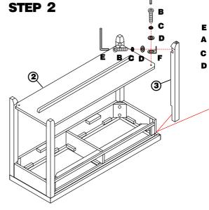
NOTE: DO NOT TIGHTEN ALL THE BOLTS UNTIL THEY ARE INSTALLED IN CORRESPONDING HOLES!
