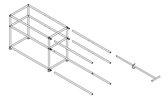
Add the connector to the sphere and insert the pole, then install pole to connector using N1. NOTE the holes of the poles need to align the holes of panel.
