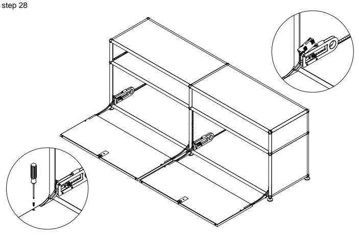
Align the slot of the door panel and insert it.
