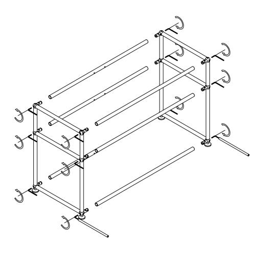
Insert the poles to the connector and install it using N3 & N5, NOTE the holes of the poles need to align the holes of panel.
