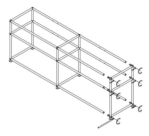
Insert the poles to the connector and install it using N3 & N5, NOTE the holes of the poles need to align the holes of panel.
