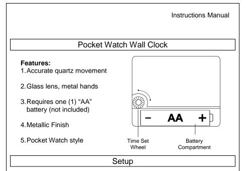
Step 1: Insert 1 fresh AA, LR6 1.5 volt ALKALINE battery according to the polarity markings. The battery is a snug fit.
