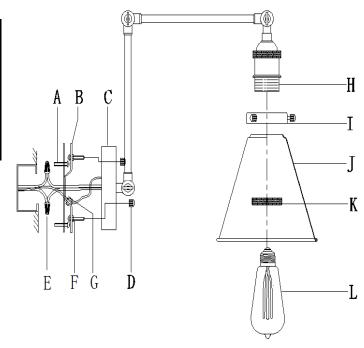
PLEASE USE ON/OFF TYPE"A" BULB MAX 40-WATT OR CFL BULB MAX 13-WATT OR LED BULB 9-WATT
