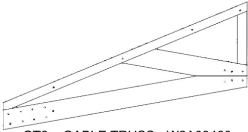
GT2 GABLE TRUSS - W2A03463 (x2) 1 3/8"x34"x64 5/8" (36x864x1640)
