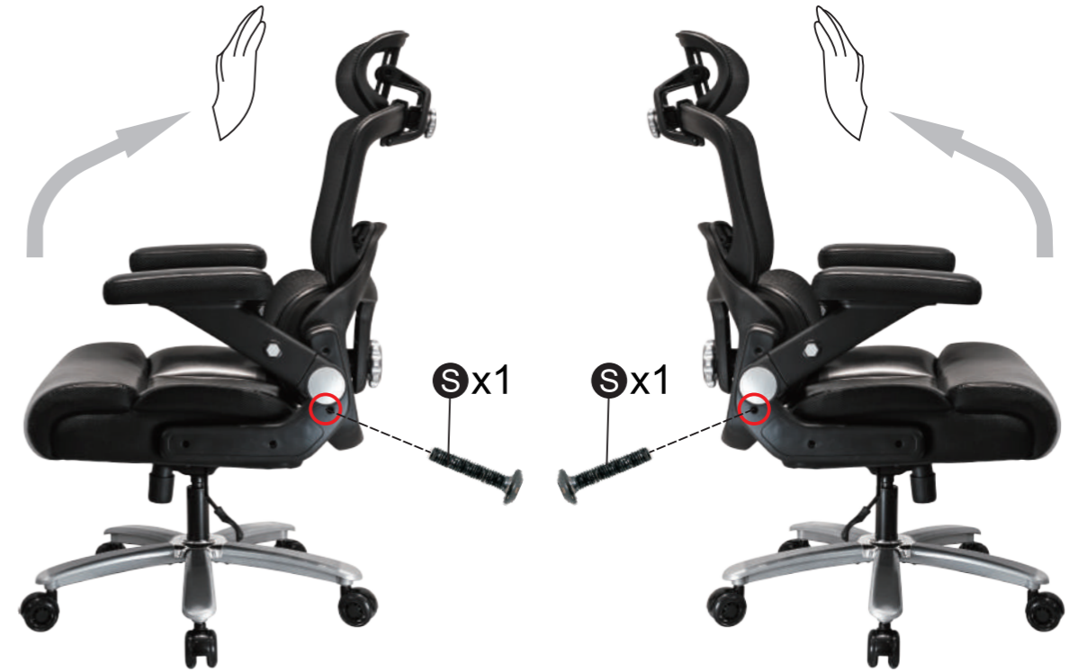
Pull up the Backrest. Use Hexagonal Bolts S to connect Backrest and Seat. (Install the lower screw holes and finally tighten all screws)
