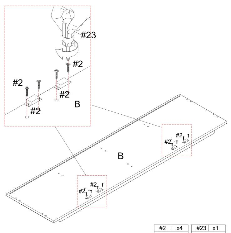
Connect the part B the pre-assembled unit in step 7.
