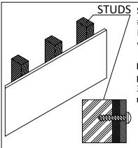
STUDS:Secure to wall with #10 x 3" screws at stud location. Locate at least 2 wall studs
