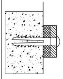
**CONCRETE:** Drill  $\frac{1}{4}$  "holes, insert #10 wall anchors and secure to wall with #10 x3" screws.
