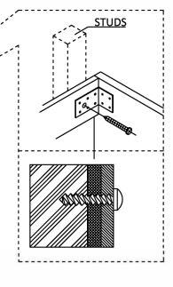
**WARNING:**INSTALLATION METHOD OF FLOATING VANITY HAS BIG RELATION WITH THE WALL STRUCTURE.
