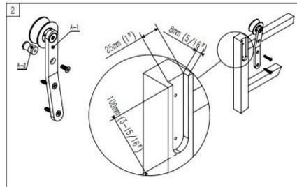
Slot the ladder according to the shape of roller. Dimensions as per  $\operatorname{\mathsf{Diagram}}$  .
