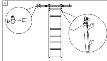
Hang the ladder onto the track and install the anti-jump pin (A-2) .Adjust the position of the stopper and fix it with a hex wrench. Then press the end cap on.
