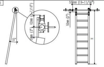
The length between two center bracket is 500mm (19 11/16")
