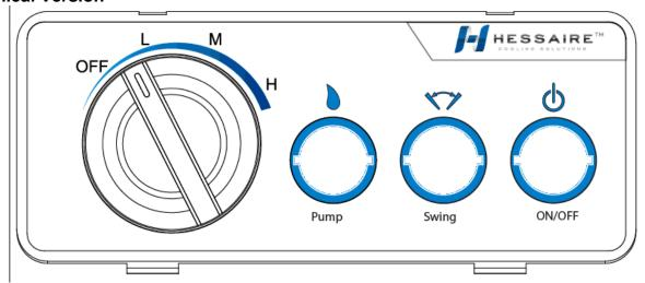
Rotary Switch/Motor Speed Has 4 positions. (Clockwise from OFF)
