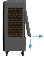
Pull out the bottom of the back panel then take it down.
