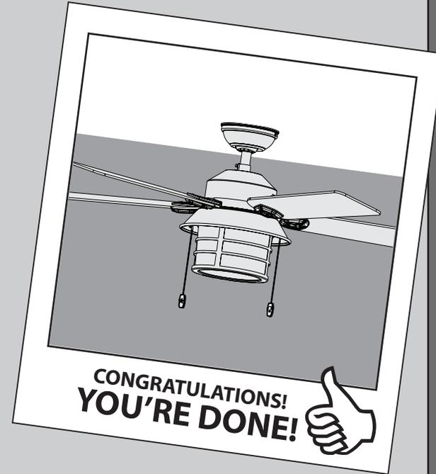
Make sure the globe assembly is securely attached to the switch housing. Failure to properly secure all three assembly screws could result in the light fixture falling.
