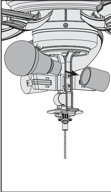
Install the included LED bulbs into the sockets. When necessary, replace with bulbs of same wattage.
