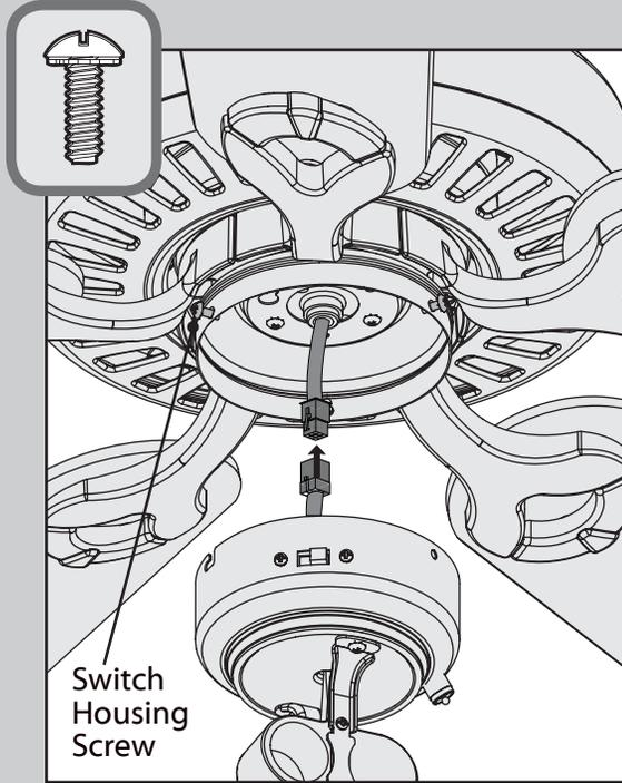
Partially install two of the switch housing screws found in the
