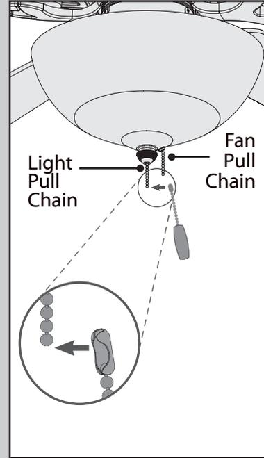
Remove the plastic break away connector. Connect the appropriate pull chain pendant to each of the short chains coming from the finial and finial cap. The fan pull chain controls the speed: from high to off. The light pull chain controls the light fixture: on and off.
