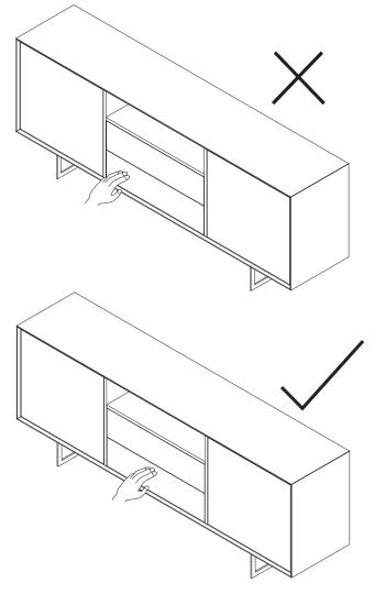
During assembly, hand tighten screws only. When the screws are in place, tighten completely.
