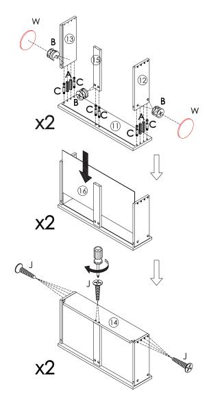
During assembly, hand tighten screws only. When the screws are in place, tighten completely.
