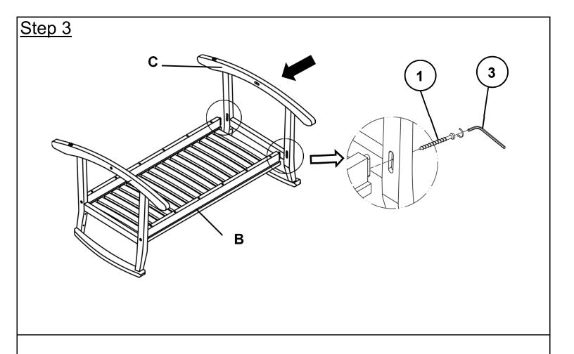
With the help from your partner, place the assembled part on step 2 to the Left Leg Panel (C) as shown in picture above.
