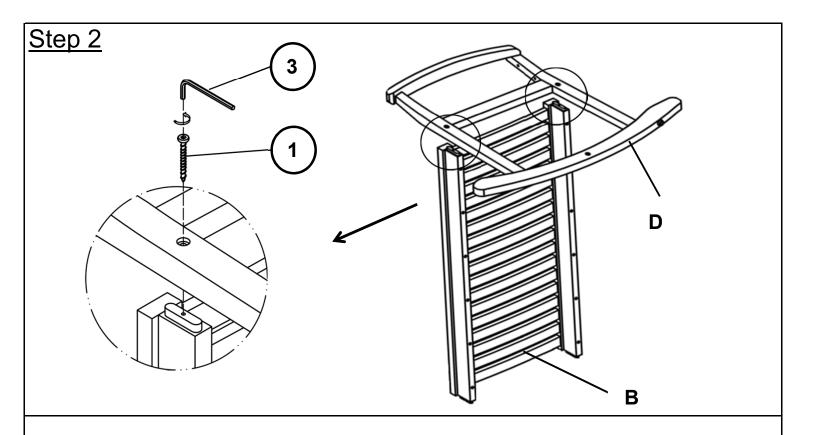
With the help from your assistance, place the Seat Panel (B) with its one side face skywards onto a clean, soft surface to avoid any scratches or damages to the product. Align the tenon of Seat Panel (B) into the Mortise of Right Leg Panel (D) as shown above. Then, affix the Seat Panel (B) with Right Leg Panel (D) by using Screws (1) and Allen Key
