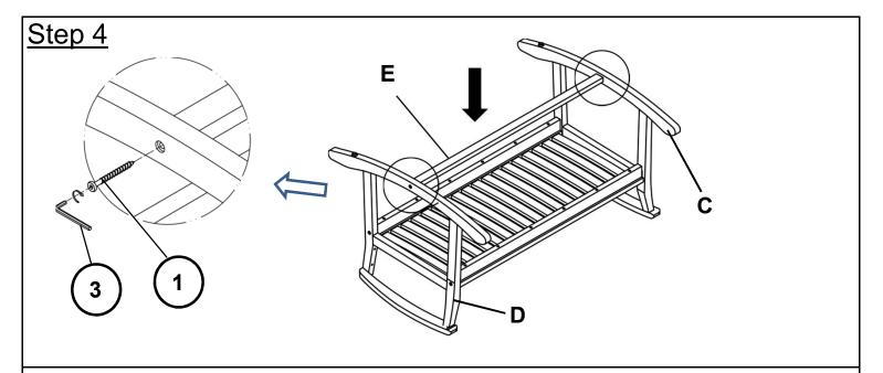
Attach the Leg Support Bar (E) to the Right Leg Panel (D) and Left Leg Panel (C) by using Screws(1) with Allen Key(3).
