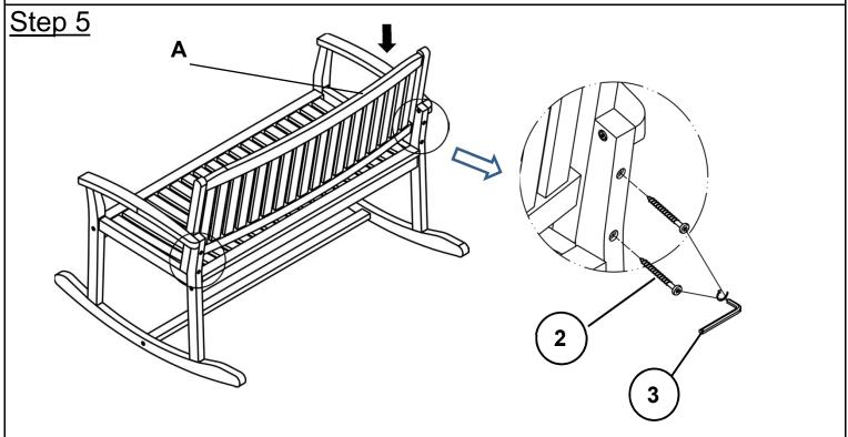
With the help from your partner, turn the finished part in step 5 right side up. Attach Backrest Panel (A) to Right Leg Panel (D) and Left Leg Panel (C), secure by using Screw (2) and Allen Key (3)
