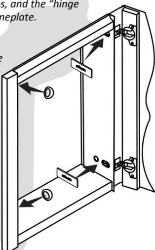
**8** The height of the shelves can be adjusted in 1/2" (13 mm) increments.
