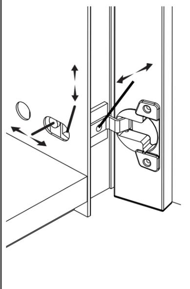
**7** Cover screws with the caps, and the "hinge adjust holes" with the nameplate.
