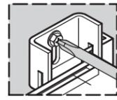
Secure with screws provided with the anchors.
