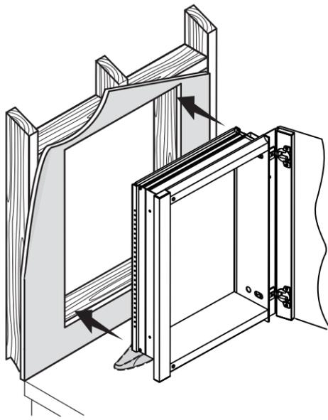
**5** Level, then secure the cabinet with 1-1/2" screws through the mounting holes and into the framing studs.
