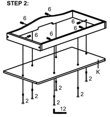
Insert Barrel Nuts (#6) into Top Front Panel, Top Back Panel and Top Side Panels before inserting Bolts (#2) from the underside of Top Panel (K). Tighten firmly with Wrench (#12).
