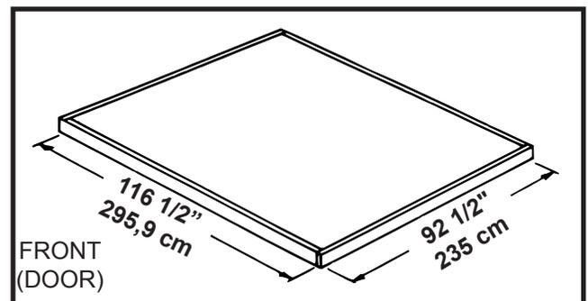
Note: Finished Slab dimensions, with lumber removed.
