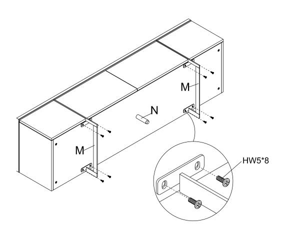
STEP10 assemble the metal legs and supporting legs
