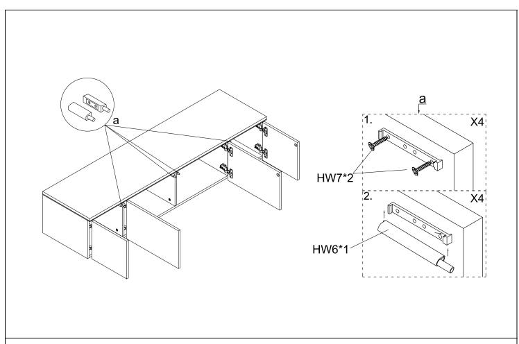
STEP9 assemble the push to open mechanism
