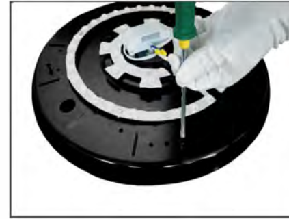
Step 4. Remove the main engine chassis screws.
