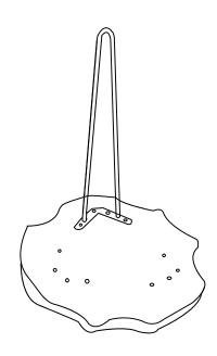
Line up one leg at a time to the holes in the mounting plate or marked lines.
