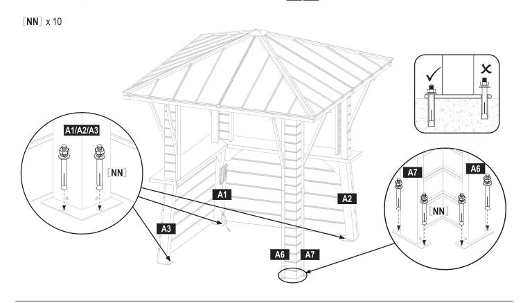
Outdoor Structure anchoring guide for anchoring gazebo to wood or concrete: If step 28, on page 14 in the assembly instructions is not properly completed, this will void the warranty.
