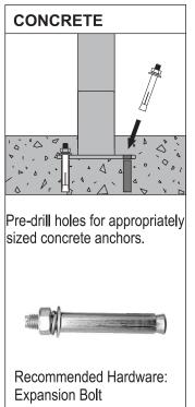
If digging for foundation, please double check for possibility of any underground utilities such as gas, telephone, cable or sprinkler lines. Refer to your local building and city codes, ordinances, neighborhood covenants, or height restrictions regarding this type of structure for guidance on acceptable installation requirements.
