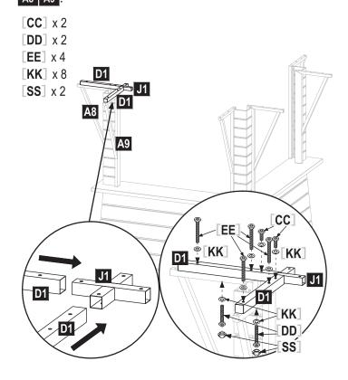
STEP 11 Slide one (1) cross beam 2 D2 onto connector 1 J1 .
