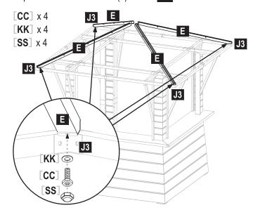
STEP 17 Use two (2) [CC] bolts, two (2) [KK] flat washers and two (2) [SS] plastic caps to attach one (1) connector 3 J3 to cross beam D3 and D4.
