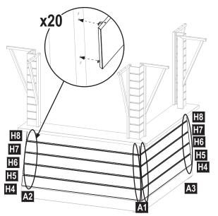
$\underline{\sf STEP~08}$  Flip the frame. Connect the decoration panel 3  $\,{\sf H3}\,$  to post  $\,{\sf A1}\,$  and  $\,{\sf A2}\,$  .
