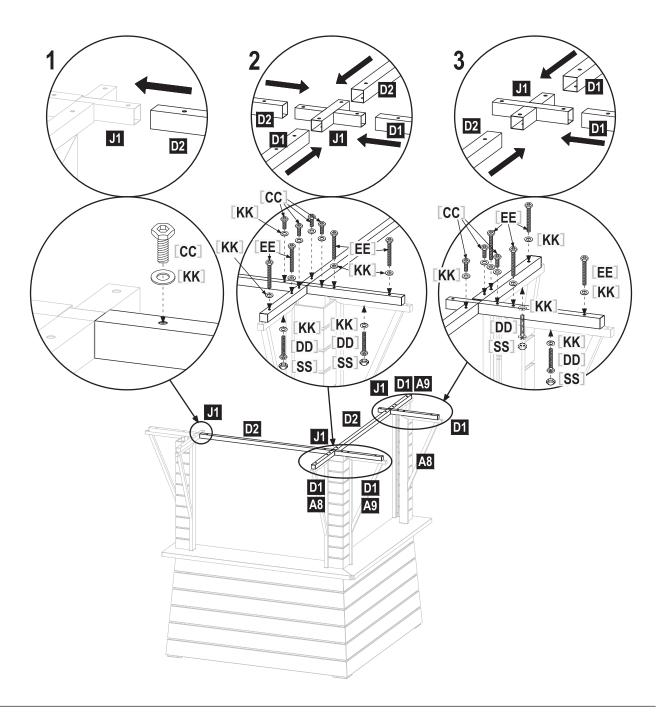
STEP 12 Slide two (2) cross beam 1 D1 onto connector 1 J1. Use two (2) [CC] bolts, four (4) [EE] bolts, two (2) [DD] bolts, eight (8) [KK] flat washers and two (2) [SS] plastic caps to attach cross beam assembly D1 J1 to post assembly A4 A5.
