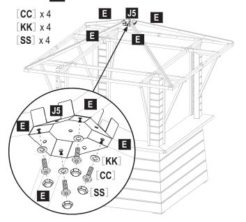
STEP 20 Use four (4) [CC] bolts, four (4) [KK] flat washers and four (4) [SS] plastic caps to attach one (1) connector 5 J5 to middle cross beams F1.
