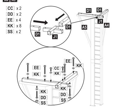
STEP 14 Use four (4) [CC] bolts, four (4) [KK] flat washers and four (4) [SS] plastic caps to attach one (1) connector 7 J7 to cross beam D1 and D2.
