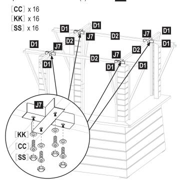
STEP 13 Slide two (2) cross beam 2 D2 onto connector 1 J1.
