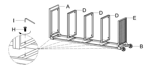
2 Attached side frame-RSF(C) with bolts(H) by allen wrench(I).
