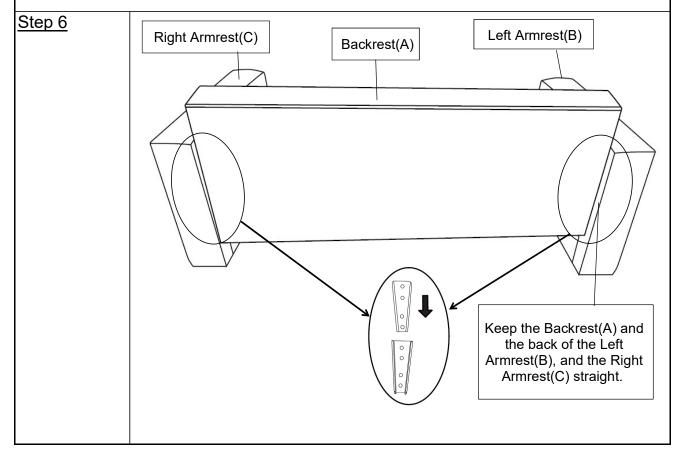
Slide the Tapered Connectors on the Backrest(A) into the Tapered Connectors on the Left Armrest(B) as shown in the picture.
