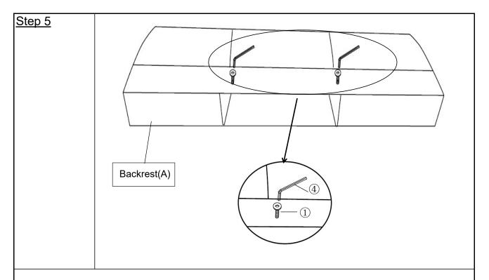
Turn the 2 Bolts( $\odot$ ) clockwise with the Allen Wrench( $\odot$ ), turn about 0.5inches (half an inch) into the Backrest(A), as shown above.
