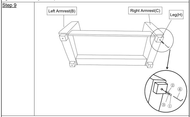
Install the Leg(H) to the Left Armrest(C) using a Bolt( $\oplus$ ),a Spring Washer Ring( $\oplus$ ),a Flat Washer Ring( $\oplus$ ),with the Allen Wrench( $\oplus$ ) turning clockwise until tight. Repeat the same step with the remaining Legs(H).
