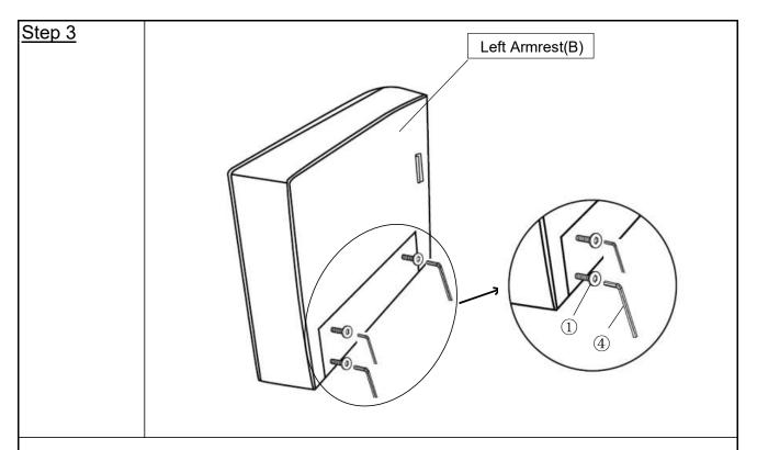
Turn the 3 Bolts(0) clockwise with the Allen Wrench(0), turning about 0.5 inches (half an inch) into the Left Armrest(B), as shown above.
