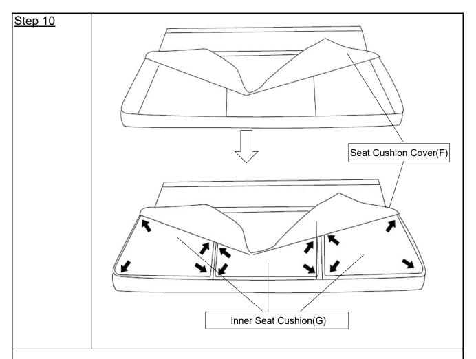
Open the zipper on the bottom of the Seat Cushion Cover(F). Put the 3 Inner Seat Cushions(G) into the Seat Cushion Cover(F) and smooth out the Seat Cushion Cover(F) as shown above.
