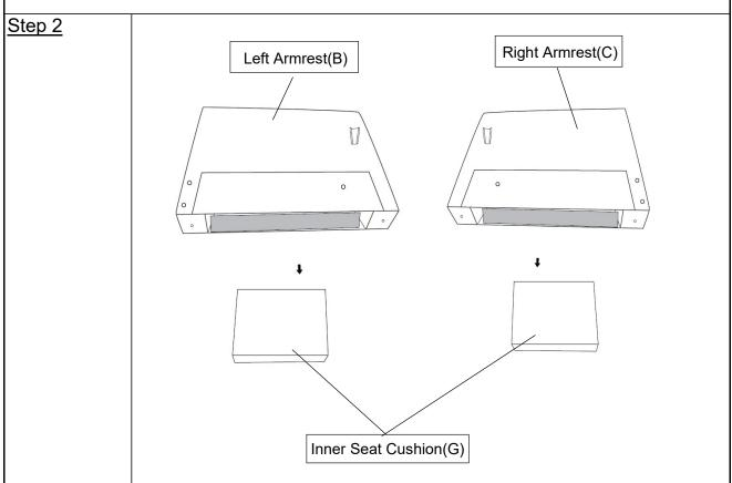
Place the Left Armrest(B) and the Right Armrest(C) face up on a clean,non-marring surface. Remove the Inner Seat Cushion(G) from the bottom of the Left Armrest(B) and the Right Armrest(C) as shown above.
